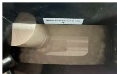
Brine Tank with water level 1/3 higher
