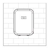
1. Using the hole positions on the back of the box as a guideline, mark two corresponding points on the wall 15 cm apart
