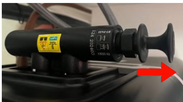
In-Service Mode: Piston Open Image 16
